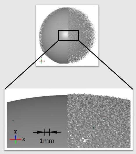
figure: Surface comparison AESUB blue and Cyclododecane
